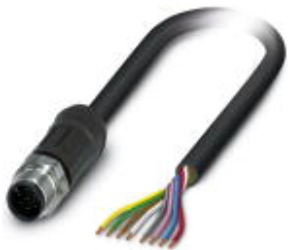
Sensor/Actuator cable, 8-position, PE-X halogen-free, black-gray RAL 7021, Plug straight M12, A-coded, on free cable end, Cable length: 2 m, for outdoor applications, with high-grade steel knurl
