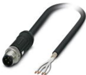
Sensor/Actuator cable, 4-position, PE-X halogen-free, black, shielded, Plug straight M12 SPEEDCON, A-coded, on free cable end, Cable length: 2 m, For railway applications
