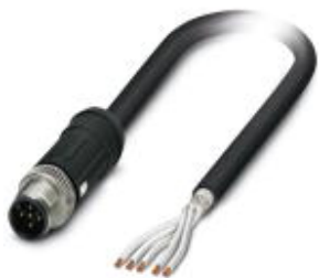
Sensor/Actuator cable, 5-position, PE-X halogen-free, black, shielded, Plug straight M12 SPEEDCON, A-coded, on free cable end, Cable length: 5 m, For railway applications
