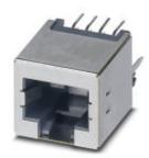
RJ45 socket insert, Type: RJ45, IP20, Degree of protection: IP20, Number of positions: 8, CAT5, Material: Copper alloy, Connection method: Solder connection
