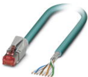
Assembled Ethernet cable, shielded, 4-pair, AWG 26 stranded (7-wire), RAL 5021 (sea blue), RJ45 connector/IP20 to free cable end, line, length 5 m
