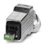
Push-pull connector (version 14), die-cast zinc, with RJ45 connector insert, 8-pos., with IDC fast connection technology, for 1 and 7-wire cores, 26 ... 24 AWG, for cable diameter of 5.5 mm ... 10 mm, cable outlet at the bottom
