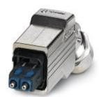
Push-pull connector (version 14), die-cast zinc, with SC-RJ insert for POF, for cable diameter of 5.5 mm ... 10 mm, cable outlet at the bottom
