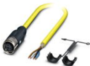
Sensor/Actuator cable, 4-position, PVC, yellow, shielded, free cable end, on Socket straight M12 SPEEDCON, A-coded, Cable length: 5 m
