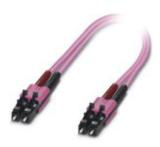
Assembled FO cable, zip cord cable, multi-mode fiberglass 50/125  $\mu$ m, OM4, plug: LC/LC, degree of protection: IP20, for installation in cable ducts or control cabinets, length: 1 m
