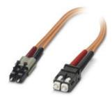
Assembled FO cable, zip cord cable, multi-mode fiberglass 50/125  $\mu$ m, OM2, plug: LC/SC-RJ, degree of protection: IP20, for installation in cable ducts or control cabinets, length: 1 m
