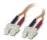
Assembled FO cable, zip cord cable, multi-mode fiberglass 50/125  $\mu$ m, OM2, plug: SC duplex/SC duplex, degree of protection: IP20, for installation in cable ducts or control cabinets, length: 1 m
