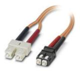
Assembled FO cable, zip cord cable, multi-mode fiberglass 50/125 µm, OM2, plug: SC duplex/SC-RJ, degree of protection: IP20, for installation in cable ducts or control cabinets, length: 1 m
