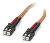
Assembled FO cable, zip cord cable, multi-mode fiberglass 50/125 µm, OM2, plug: SC-RJ/SC-RJ, degree of protection: IP20, for installation in cable ducts or control cabinets, length: 1 m
