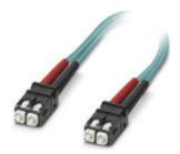
Assembled FO cable, zip cord cable, multi-mode fiberglass 50/125  $\mu$ m, OM3, plug: SC-RJ/SC-RJ, degree of protection: IP20, for installation in cable ducts or control cabinets, length: 1 m
