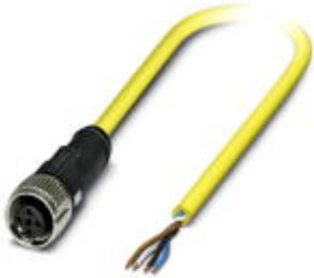
Sensor/Actuator cable, 4-position, TPE, yellow RAL 1021, free cable end, on Socket straight M12 SPEEDCON, A-coded, Cable length: 5 m
