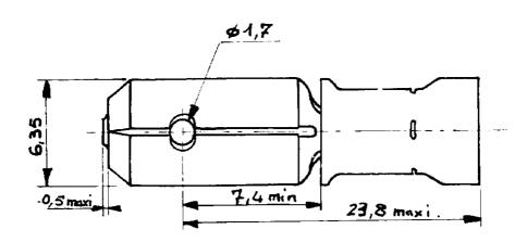
C 1948BY AMP INCORPORATED, ALL RIGHTS DESSIN CLIENT RESERVED. AMP PRODUCTS COVERED BY UNIQUEMENT POUR RÉFÉRENCES PATENTS AND/OR PATENTS PENDING MATIÈRE ET FINITICN Laiton 1/2 dur DE FRANCE PONTOISE SERIE 6,35 27 | 2 | 93 changed hole Shape FB - 2 étamé ß DIMENS-FILD ISOLANT 5\_11.71 4 à 6 mm Wait 2,6 à 6,6 PI.D.G TOLERANCES SAUF INDICATION ± 0.3 ±5° VER DATE CHANGEMENT 2141085 IND APPROUVE DESSINE دعل 5-11-68 LANGUETTE FASTON PLAG VERIFIE
