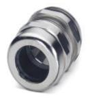
Cable gland, cable gland material: Nickel-plated brass, external cable diameter 5 mm ... 9 mm, shielding: yes, connecting thread: M16 x 1.5, color: silver, with O-ring
