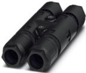
QUICKON H-distributor, black, 4+PE-pos., 2.5 mm² ... 6.0 mm²/690 V/40 A, for cable diameter of 12 mm ... 20 mm, with a sealing bolt.
