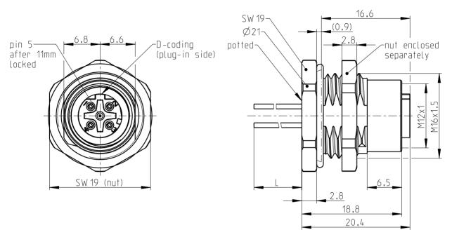
All specified data refers to the mounted M12 installation plugs  $\geq$  IP54 and requires that the connector pair be correctly plugged and locked. Influences from wires, cables or PCB mounting are also to be taken into consideration.
