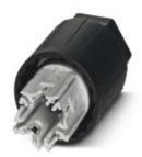
QUICKON nut, black, 4+PE-pos., 1.0 mm<sup>2</sup> ... 2.5 mm<sup>2</sup>/690 V/20 A, for cables with 9 mm ... 16 mm diameter.
