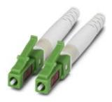
LC duplex connector, with long bend protection, for single mode  $9/125 \mu m$ , APC polishing (8°), green, value pack: 10 pcs
