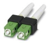
SC duplex connector, with long bend protection, for single mode 9/125 μm, APC polishing (8°), green, value pack: 10 pcs
