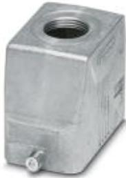
Sleeve housing B10, for single locking latch, Material: Die-cast aluminum, salt water resistant, Cable outlets: 1, straight, Height: 57 mm, Cable gland: none, Gland: no, 1x M20, Standard
