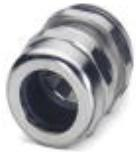
Cable gland, Cable gland material: Brass, nickel-plated, External cable diameter 9 mm ... 13 mm, Shielding: yes, Connecting thread: M20, Color: silver
