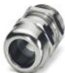
Cable gland, Cable gland material: Brass, nickel-plated, External cable diameter 19 mm ... 28 mm, Shielding: No, Connecting thread: M40, Color: silver
