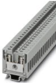
Feed-through terminal block, Connection method: Screw connection, Cross section: 0.2 mm 2 - 4 mm 2 , AWG 24 - 12, Width: 5.2 mm, Color: gray, Mounting type: NS 15
