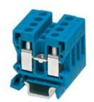
Mini feed-through terminal block, nom. voltage: 250 V, nominal current: 24 A, connection method: Screw connection, number of connections: 2, cross section:0.2 mm² - 2.5 mm², AWG: 24 - 14, width: 5.2 mm, color: blue, mounting type: NS 15
