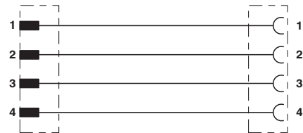
Contact assignment of the DEUTSCH connectors
