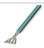
CAT6a-S/STP cable, 4 x 2 x 23 AWG, solid (1-wire), shielded, outer sheath: Halogen-free PUR, outside diameter 8.0 mm, RAL 5021 (water blue), cable ring 100 m
