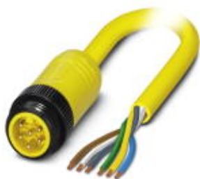
Power cable, 6-position, PVC, yellow, Plug straight 7/8"-16UNF, A - standard, on free cable end, cable length: 1 m
