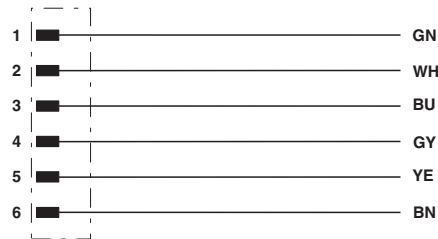
Contact assignment of 7/8" plug
