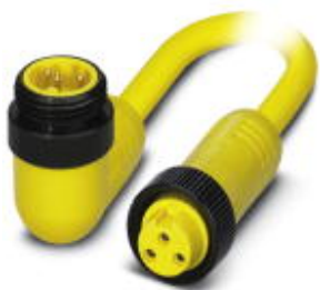
Power cable, 3-position, PVC, yellow, Plug angled 7/8"-16UNF, A - standard, on Socket straight 7/8"-16UNF, cable length: 1 m
