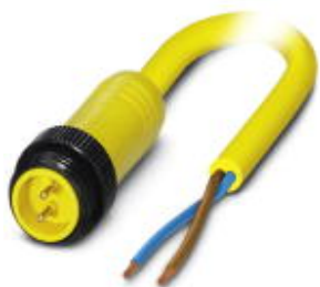
Power cable, 2-position, PVC, yellow, Plug straight 7/8"-16UNF, A - standard, on free cable end, cable length: 2 m
