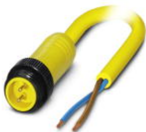
Power cable, 2-position, PVC, yellow, Plug straight 7/8"-16UNF, A - standard, on free cable end, cable length: 10 m
