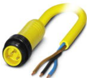
Power cable, 3-position, PVC, yellow, Plug straight 7/8"-16UNF, A - standard, on free cable end, cable length: 5 m
