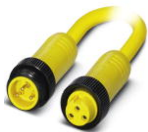
Power cable, 3-position, PVC, yellow, Plug straight 7/8"-16UNF, on Socket straight 7/8"-16UNF, cable length: 2 m
