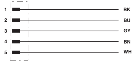
Contact assignment of 7/8" plug
