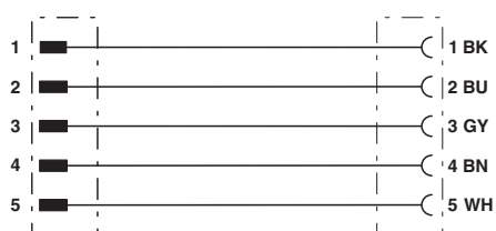
Contact assignment of 7/8" plugs/sockets
