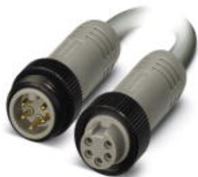
Bus system cable, DeviceNet™, 5-position, PVC, gray, Plug straight 7/8"-16UNF, on Socket straight 7/8"-16UNF, cable length: 2 m
