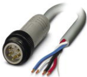
Bus system cable, DeviceNet™, 5-position, PVC, gray, Plug straight 7/8"-16UNF, on free cable end, cable length: 2 m
