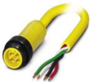
Power cable, 4-position, PVC, yellow, Plug straight 7/8"-16UNF, A - standard, on free cable end, A - standard, cable length: 5 m
