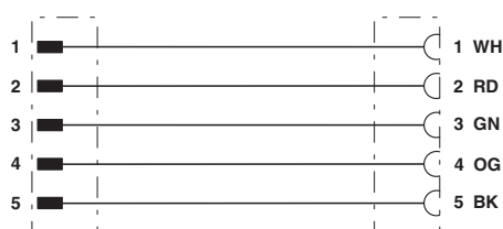
Contact assignment of 7/8" plugs/sockets
