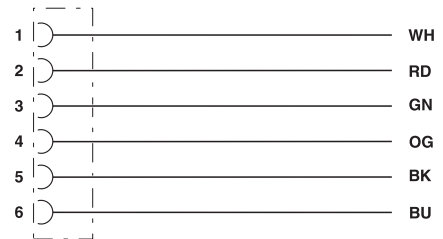
Contact assignment of 7/8" socket
