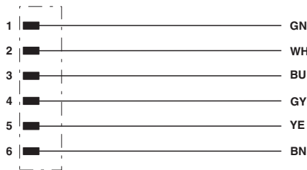
Contact assignment of the 7/8" plug
