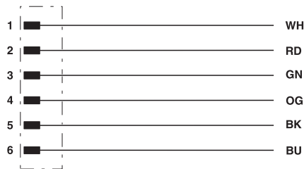
Contact assignment of the 7/8" plug
