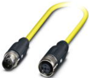
Sensor/Actuator cable, 3-position, PVC, yellow RAL 1021, shielded, Plug straight M12 SPEEDCON, A-coded, on Socket straight M12 SPEEDCON, A-coded, Cable length: 15 m
