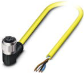
Sensor/Actuator cable, 4-position, PVC, yellow RAL 1021, free cable end, on Socket angled M12 SPEEDCON, A-coded, Cable length: 20 m
