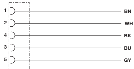
Contact assignment of the M12 socket
