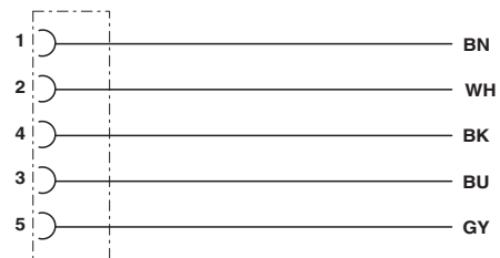
Contact assignment of the M12 socket
