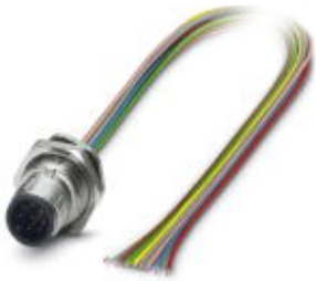
Sensor/actuator flush-type plug, 8-pos., M12 SPEEDCON, rear/screw mounting with M16 thread, with 0.5 m TPE litz wire, 8 x 0.25 mm 2
