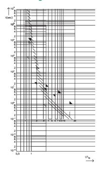
FI = 1.25 (max. operating current:  $0.8 \times I_{rat}$  at  $23^{\circ}$ C)
