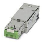
RJ45 connector, contact inserts: x , degree of protection: IP20, number of positions: 8, 1 Gbps, CAT5 (IEC 11801:2002), material: Zinc die-cast, connection method: IDC fast connection, connection cross section: AWG 23- 22, cable outlet: straight
